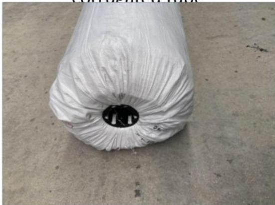
4.Insert the retainer to make the package stronger and prevent the carpet from leaking out.
