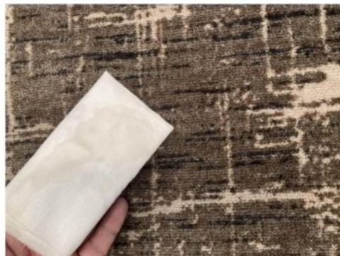
Wet tissue friction test
