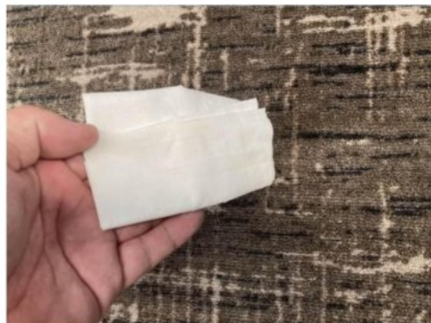
Dry paper towel friction test
